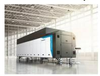
Some of you might be asking, what is a tunnel washer? A tunnel washer is a long metal tunnel with multiple pockets. Each pocket will contain 250 lbs. of soiled product and as the product moves from one pocket to the next, the product will become cleaner the further along it moves in the process. Pictured to the left is a tunnel washer and to watch a video of it in action, click here <a href="https://www.youtube.com/watch?v=Ys1ll8hq5VI">https://www.youtube.com/watch?v=Ys1ll8hq5VI</a>
