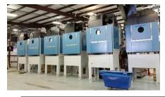
We will have multiple conveyors to move clean product to the dryers or to a lift station. To start, we will be installing 5 highly efficient dryers (pictured left). To watch a video of how the dryers work, click the link below <a href="https://www.youtube.com/watch?v=wyGvS5fbu9k">https://www.youtube.com/watch?v=wyGvS5fbu9k</a>. We will also be adding additional overhead storage for clean product in the new addition.
